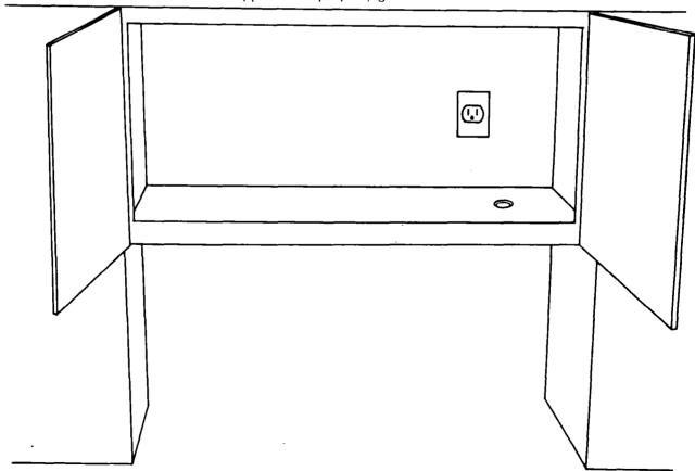
The power supply cord and plug must be connected to a separate AC 120-Volt, 60 Hz, 15 or 20 Amp. branch circuit, single grounded receptacle. The receptacle should be located inside the cabinet directly above the Microwave/Hood System mounting location.
